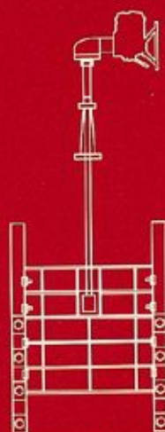
MX/B320 mounted to sluice gate
