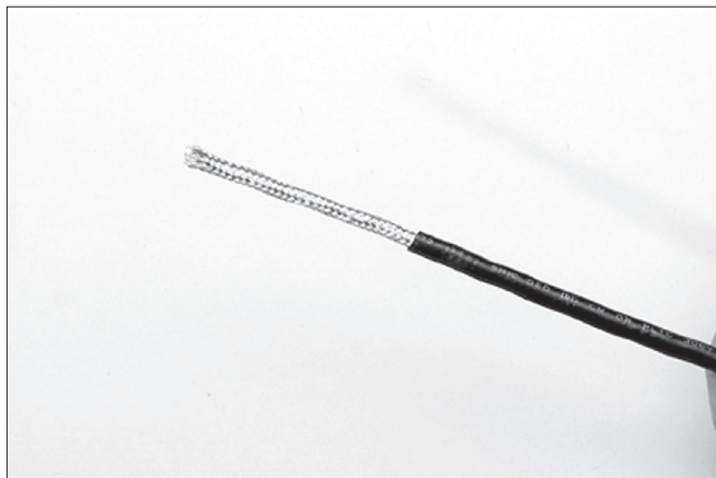
Figure 3.8 – Removing outer plastic jacket
